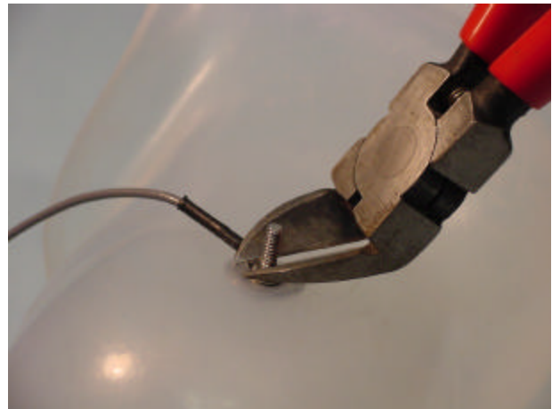
Fig. 5 – Cut off excessive stud length
