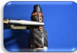
6. Apply final layer of carbon fiber to mold. Pull a final vinyl glove finger over model and heat in over under vacuum for 3 hours
