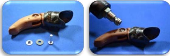
9. Install spring. Insert spring into fingertip and secure with 0-80 X 1/2 inch screw provided. Loop sewing thread through spring loop and guide both ends of thread through hole in finger base and exit both out of the top of the finger base. Pull back on both ends of thread to pull spring loop into screw hole. Insert 0-80 X 3/8 inch screw provided into hole to secure spring
