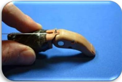
10. Install cable assembly. Route both ends of cable through top of finger base and into fingertip. Pull cables out of hole using tweezers provided. Set cable length so the silicone sleeve is positioned over the knuckle. Tie two knots in cable and superglue knot. Cut off excess cable and pull knot into hole. Secure in place with set screw provided
