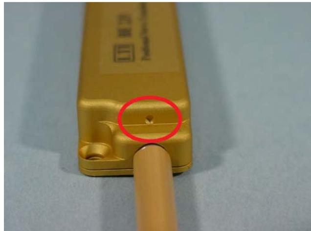
Figure 4 – Drill Hole for Rerouting Spectra Cord - 1” Travel
