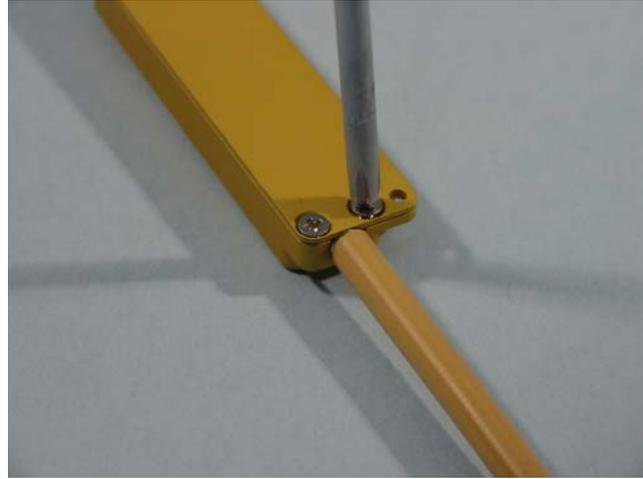
Figure 6 – Securing the End of the Bowden Cable
