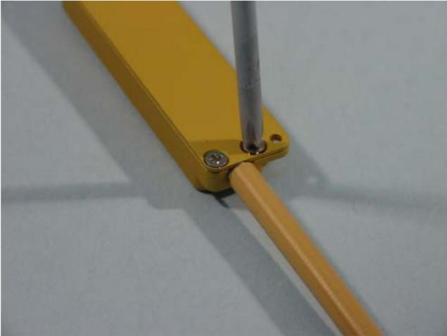
Figure 5 – Securing the End of the Bowden Cable
