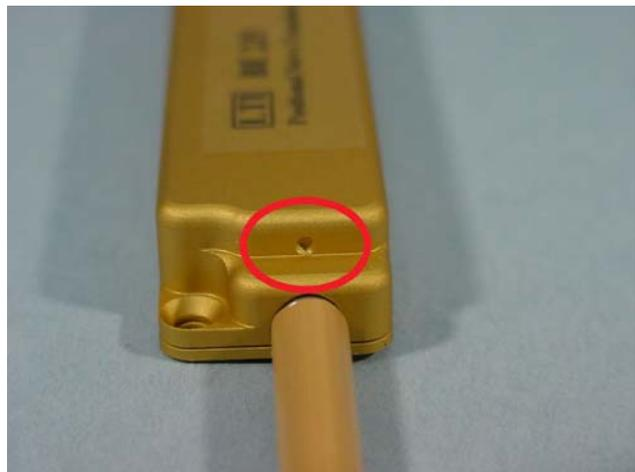
Figure 4 - Drill Hole for Rerouting Spectra Cable - 1" Travel
