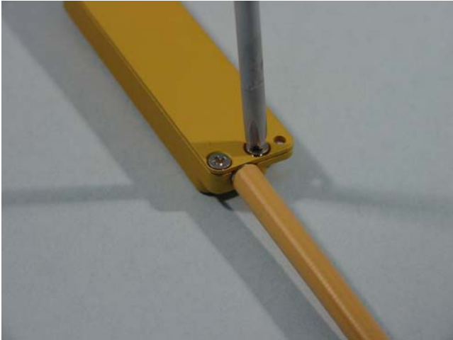
Figure 5 – Securing the End of the Bowden Cable
