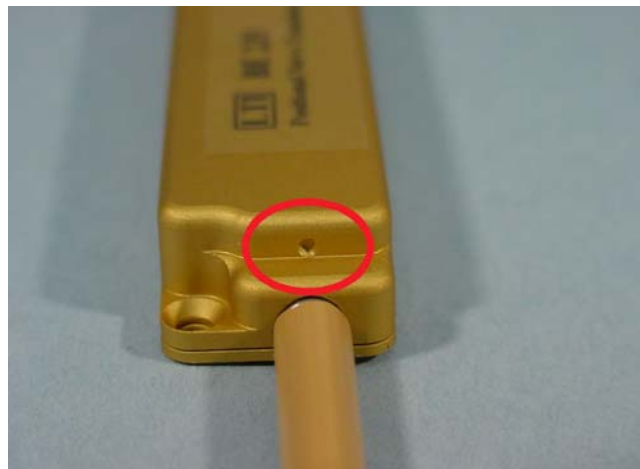
Figure 4 - Drill Hole for Rerouting Spectra Cable - 1" Travel
