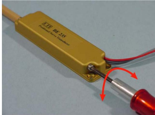
Figure 6 - Spring Tension Adjustment
