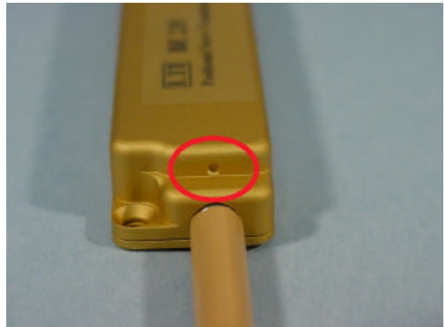
Figure 4 – Drill Hole for Rerouting Spectra Cable - 1” Travel
