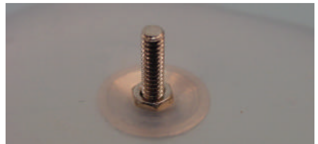
Nut squeezing liner down into the cavity
