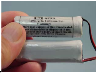
Fig 2 – BP88 Split-cell Li-ion Battery
