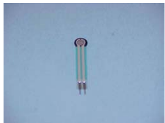
TP04 Single \frac{1}{4} " diameter Touch Pad with solder tabs, no connector
