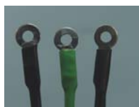
VGC625 One Remote Myoelectrode-Amplifier for VG III VGC626 Two Remote Myoelectrode-Amplifiers for VG III Separate Ring terminals are supplied for use with 4-40 studs on EL01 or EL02 metal electrodes.
