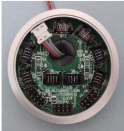
Fig. 7. Single myoelectrode.
