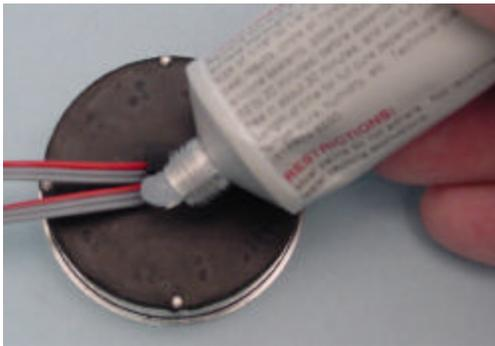
**Figure 3.** Seal the hole where the wires pass through the rubber backing. Use silicone tub seal or equivalent.
