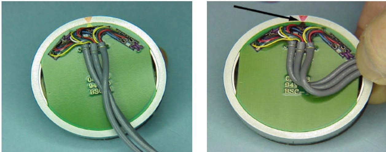
**Figure 5.** The photo on the left shows a simple twist in all three wires on the Cover Board. The photo on the right shows what happens when the board is rotated. The twist avoids having the wires bunch up during humeral rotation. A mark (see arrow) may be added to assist in aligning the Cover Board and Input Board.
