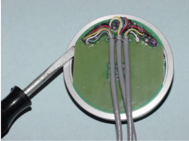
**Figure 6.** Carefully pry the Cover Board from the Input Board assembly. Pry first on one side and then on the other to avoid bending the connector pins.
