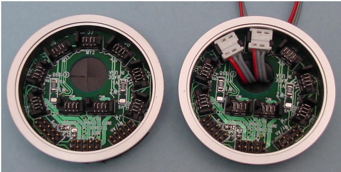
**Figure 1. Making connections to the Input Connector Board.** On the left you can read the labels MY1 and MY2. On the right, the connectors from the preamplifiers are passed up through the rubber seal and pushed in place. The wires block further view of the labels.
