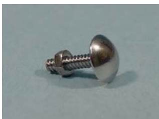
EL03 Remote Metal Electrode, Small Dome, Cavity-backed™ 0.37" (9.4mm) dia. dome rises 0.09" (2.2mm) with 4-40 threaded stud for attaching to REC ring terminal. Supplied with two small profile 4-40 nuts.
