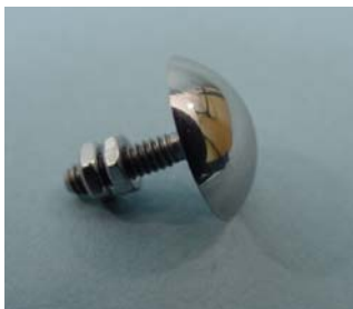
EL01 Remote Metal Electrode, High Dome, Cavity-backed™ 0.56" (14mm) dia. dome rises 0.19" (4.8mm) with 4-40 threaded stud for attaching to REC ring terminal. Supplied with two small profile 4-40 nuts.
