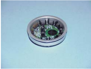
BE304 Input Connector Board, Boston Digital Arm Supplied with Boston Digital Arm (BE300)
