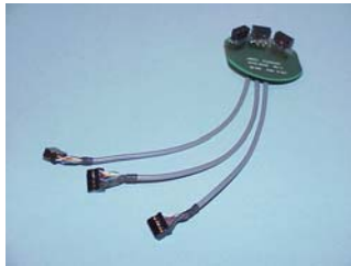
BE390 Cross Elbow Cable Set, Boston Digital Elbow Supplied with Boston Digital Arm (BE300)
