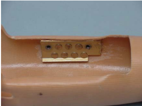
Fig. 8.1 Attachment plates cemented to each side of the Forearm.
